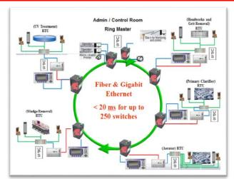
Building a ring topology redundancy Ethernet network could perform a "Self-Healing" function in order to re-build the network and route data immediately with a backup path. Typically, Ethernet switches have a built-in traditional STP/RSTP network recovery protocol but they still have a limitation for the maximum downtime (2~3 seconds); which means there's risk about some data being dropped during this period.
